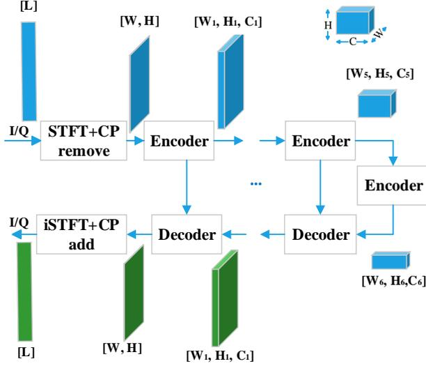
**Fig. 1.** Schematic of the interference cancellation model, detailing the input tensor’s progression. Starting with an in-phase and quadrature (I/Q) baseband RF signal, the model applies STFT and CP removal to obtain the time-frequency domain representation  $[W, H]$ . The signal is then processed through a sequence of encoders and decoders, culminating in an iSTFT with CP addition for interference mitigation.
