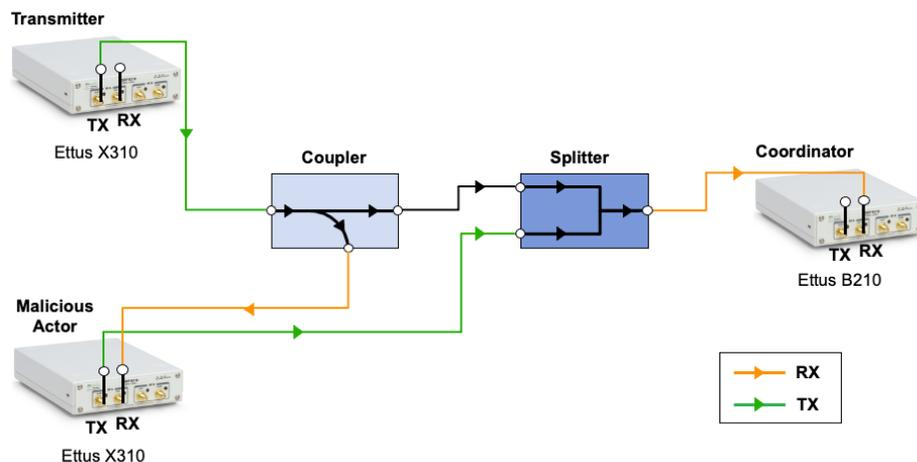
Figure 1: Wiring setup for the SDR-based signal testbed
